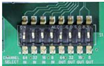
32x32: Switch 1 and 5 are switched OFF (64 ch dipswitches are off)
