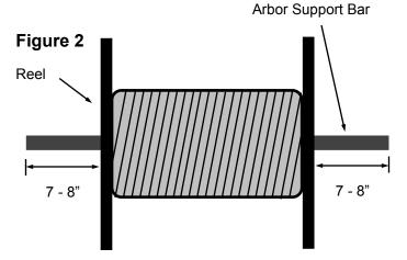
3. With reel on a flat surface - insert arbor support bar through center hole of reel. A minimum of 7 - 8" should protrude on each side of reel. (Figure 2)
