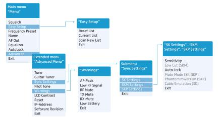
When one of the standard displays is shown on the display panel, you can get into the main menu by pressing the jog dial. The extended menu "Advanced Menu" and the other menus can be accessed via the corresponding menu items.
