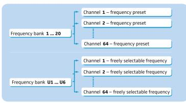
Each of the channels in the frequency banks "1" to "20" has been factory-preset to a fixed receiving frequency (frequency preset). The factory-preset frequencies within one frequency bank are intermodulation-free. These frequencies cannot be changed.
