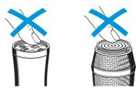
When unscrewing the microphone head ① during operation, the muting function is automatically activated. "MUTE" appears on the display panel.
