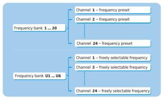
Each of the channels in the frequency banks "1" to "20" has been factory-preset to a fixed transmission frequency (frequency preset).
