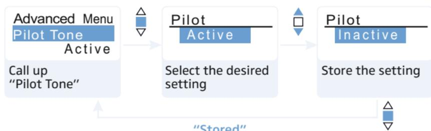
The radio microphone adds an inaudible pilot tone to the audio signal. The receiver detects and evaluates the pilot tone, and is thus able to identify the signal of the matching transmitter and mute all others. The pilot tone supports the receiver’s squelch function.
