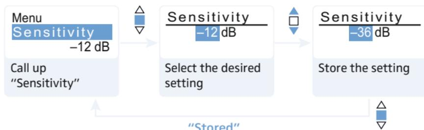
Adjustment range: 0 to -48 dB, adjustable in steps of 6 dB
