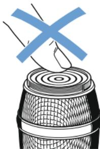
When unscrewing the microphone head ① during operation, the muting function is automatically activated. "MUTE" appears on the display panel.
