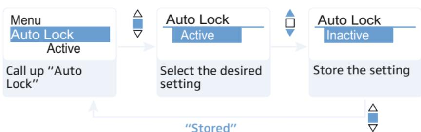
The lock mode prevents that the radio microphone is accidentally switched off or programmed during operation. The lock mode icon ⑤
