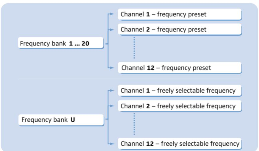
Each of the channels in the frequency banks “1” to “20” has been factory-preset to a fixed transmission frequency (frequency preset). The factory-preset frequencies within one frequency bank are intermodulation-free. These frequencies cannot be changed.
