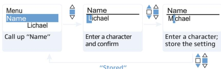
Via the "Name" menu, you can enter a freely selectable name (e.g. the name of the performer) for the radio microphone.
