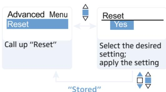
When resetting the radio microphone, only the selected settings for the pilot tone and for the frequency bank “U” remain unchanged.
