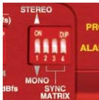
Fig 10-6: SILENCE Detect Stereo/Mono & Sync Source DIPSwitch
