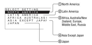
Press the ↑ or ↓ button to select the area where you intend to use the unit and press the → or ENTER button.
