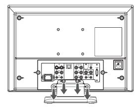
**2** Attach the unit to the rack using the mounting bracket.
