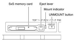
Be sure to insert SxS memory cards in the proper orientation and direction. When an SxS memory card is inserted and the unit recognizes it properly, the mount indicator lights.
