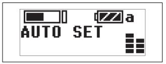
**4** Press and hold the SET button on the tuner for at least one second.
