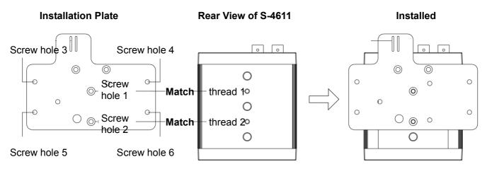
Match the screw holes 1&2 with the threads 1&2 of S-4611, and fix the installation plate to the S-4611 by the supplied screws. The screw holes 3, 4, 5, 6 are used to install S-4611 to wall or racks.
