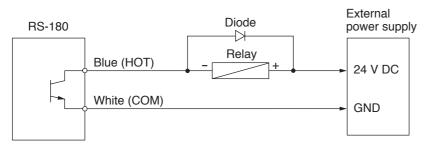
Open collector output: 24 V DC (max.), 30 mA.
