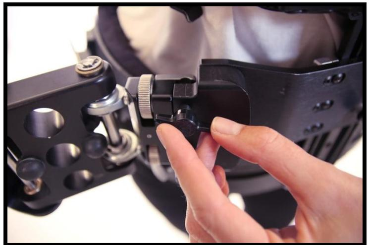
Typically, your side-to-side adjustment won't need to be changed, but if the System does move to one side, you can correct it here.
