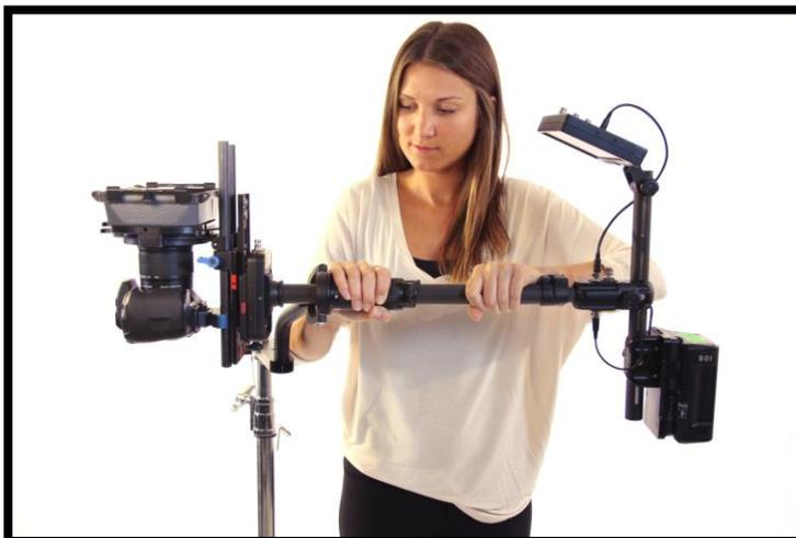
Grasp the Post, it will move freely inside the open Gimbal. Grasp the Gimbal Grip or use your thumb to push against the Gimbal, sliding the Post one way or the other until the Sled balances horizontally like a seesaw.
