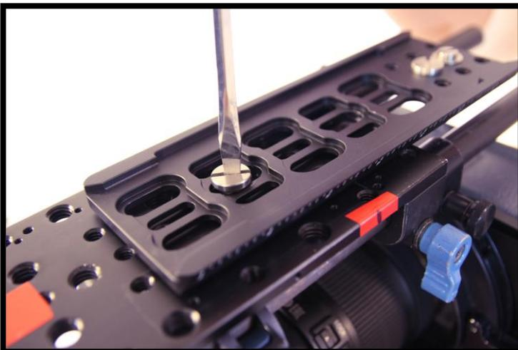
Fasten with the appropriate camera screw in the nearest opening. Do not over tighten, but ensure the camera will not rotate.
