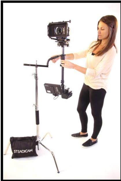
Set up the Docking Bracket on a stand and use a sand bag or a friend to keep it from toppling while the rig is on the balance pin.
