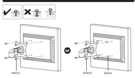
Lift the display and align the rear mounting holes with the mount assembly's VESA plate.
