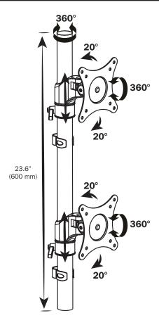
To adjust the desired location or tilt, use the appropriate Hex Key to adjust. Turn clockwise to tighten or counterclockwise to loosen.
