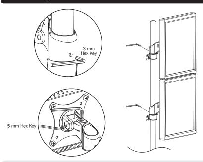
Use the appropriate Hex Keys to adjust the swivel. Turn clockwise to increase tension or counter-clockwise to reduce tension.
