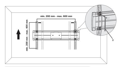
Adjust Adapter Brackets to fit VESA hole pattern on your display. Tighten all Screws. **NOTE**: Verify proper alignment of all holes.
