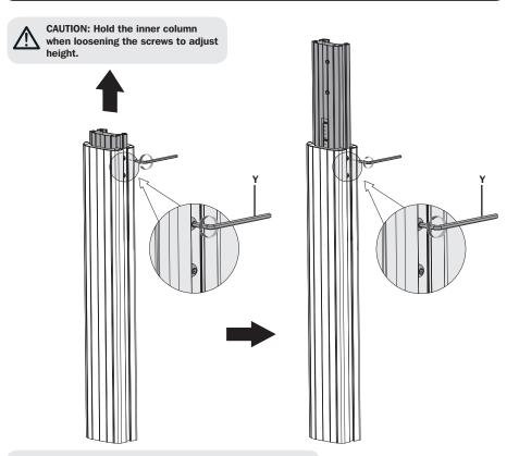
Adjust inner Column J to the desired height, then tighten all screws.
