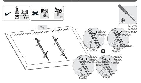
Note: Choose appropriate screws, washers and spacers (if necessary) according to the type of screen.
