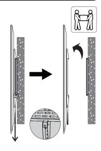
• Before releasing the display, make sure adapter brackets have been safely attached to the wall plate.
