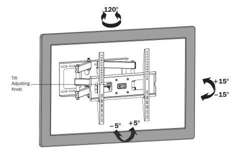
To adjust the tilt angle, loosen the Tilt Adjusting Knobs located behind the wall mount arm assembly plate. Once the display is at the desired position, retighten the knobs to hold.
