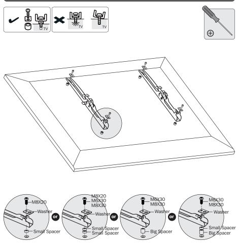
**Note:** Choose appropriate screws, washers and spacers (if necessary) according to the type of screen.
