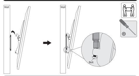
Using an assistant or mechanical lifting equipment, hook the display with attached adapter brackets over the top of the mounted wall-plate. Tighten the two bolts on the bottom of the adapter brackets to secure the unit.
