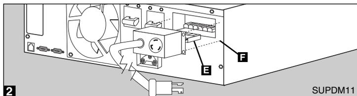
**2** Insert the connector cable from the SUPDM **E** into the connectors in the power module's terminal box until the release tab clicks in place. Screw the SUPDM into place **F**.
