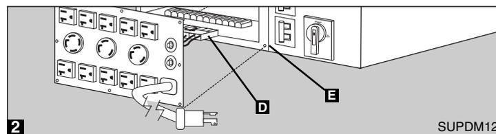
**2** Insert the connector cables from the SUPDM **D** into the connectors in the transformer module's terminal box until the release tabs click in place. Screw the SUPDM into place **E**.
