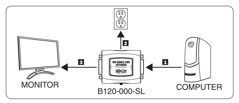
Connect the longer DVI-D Single Link cable between the source and the connector on the B120-000-SL labeled "Source."
