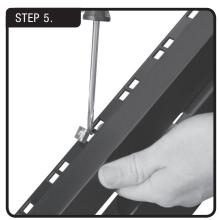
Use a flat head screw driver too attach mounting brackets. Use small screws to attach equipment to mounting brackets.
