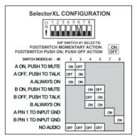
Switch 1 selects Momentary (press and hold) or Alternate (push on, push off) footswitch action.
