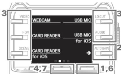
1. When the Recording Screen is open, press  **SETTING/EXIT** to open the Setting Screen.
