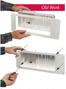
Attach trim plate to box section with (4) #8 x 3/4" (supplied) screws through these holes.
