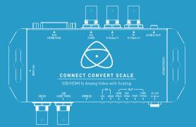
Connect 3G/HD/SD-SDI and HDMI video sources to Composite/S-Video, Analogue DVI and Component devices, with resolution and frame scaling up to 1080p60.
