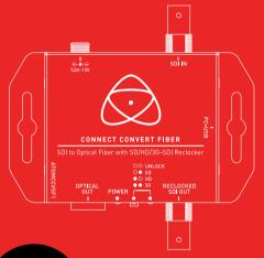
Converts SDI to Fiber for extremely long video runs exceeding the maximum length capable for SDI cable (200m) or a SDI repeater (400m).
