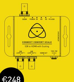
Featuring full size 3G/HD/SD-SDI, lockable HDMI, lockable DC power, removable included mounting ears and conversion/frame rate/resolution scaling up to HD 1080p60.
