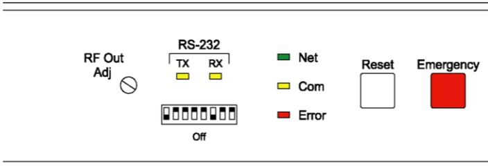
Check the front panel of the Head End, as shown above, and see if the last 3 DIP switches under the RS-232 LED are set as follows:
