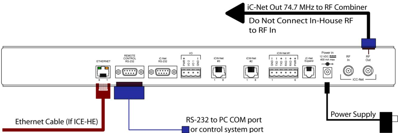
Next, connect the included RS-232 cable between the PC's 9-pin RS-232 port or USB adapter to the RS-232 Remote Control port on the back of the ICC-HE. The ICE-HE can also receive control commands via IP.
