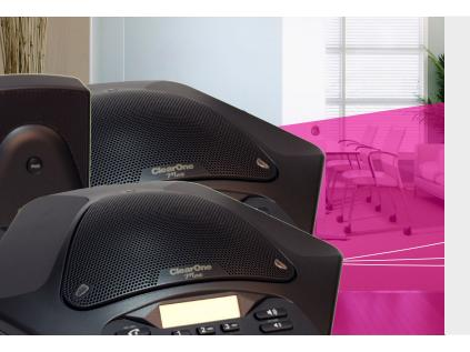
The industry's first dual-phone wireless tabletop conferencing system. MAXAttach Wireless provides expanded wireless coverage for medium-sized conference rooms, delivering clear, full-duplex audio through two complete phone units - all with no cables in the way.
