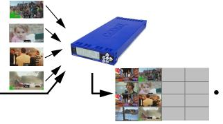
More downstream BBG-1070-QS units can be added and have its PiPs added next to those furnished from the upstream card cascade. Here, PiP insertions are arranged in columns, although almost any desired grid and arrangement scheme is possible.
