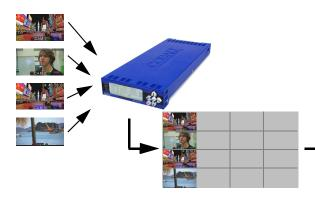
The cascade output (consisting of the four PiP images and a full-size underlay) can be sent to another BBG-1070-QS as a cascade input, serving as an underlay which can accept more PiP insertions.
