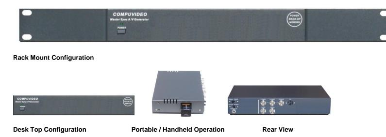
Compuvideo new Low Cost Precision Professional Black Burst Generator offers auto power back-up assuring that even if power is lost to the unit - it will still work without any interruption.
