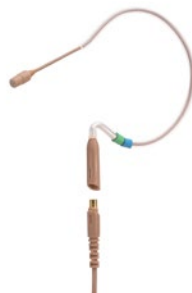
The E2 water-resistant detachable connector makes cable or transmitter changes easy.
