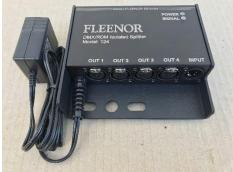
The 124 is an economical bi-directional DMX512/RDM splitter. It is available with 3 pin (model 124-3) or 5 pin (model 124-5) XLR connectors for all DMX512/RDM connections, as well as RJ45 connectors (model 124-RJ) and terminal block connectors (model 124-TB). These splitters have fully isolated inputs. The four outputs are separately driven, but are not isolated from one another.
