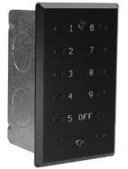
The Preset 10 Architectural is a lighting control station capable of storing up to ten presets. These presets are recorded by capturing the output of a DMX512 console. Each preset can then be assigned a unique fade time, from 0 to 999 seconds. Presets are recalled by pressing one of the buttons.
