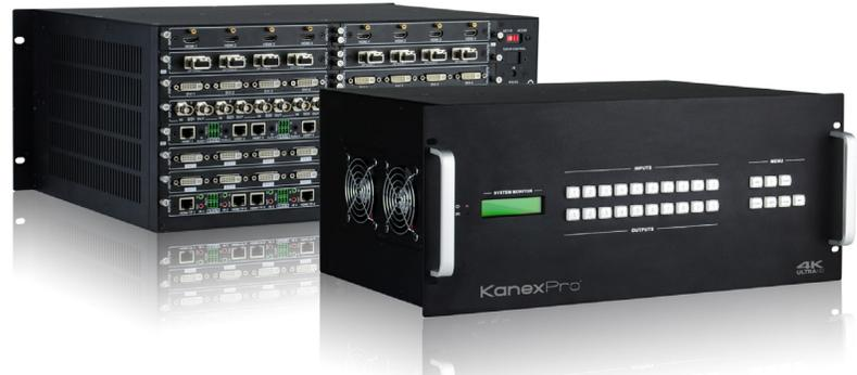
The **KanexPro HDMMX3232-4K** is a 32 input by 32 output modular matrix switcher chassis with eight input slots and eight output slots; each modular input or output card supports up to eight device connections. As an add-on to front panel control, the HDMMX3232-4K can be controlled via IR, RS232, or TCP/IP connections.
