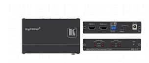
FC17 is a versatile HDMI 4K@60Hz (4:4:4/4:2:0) converter tool. FC17 can convert from 4:4:4 to 4:2:0 color sampling and offers EDID management via a userfriendly Windows application. It also enables interoperability between HDCP 2.2 and HDCP 1.4 systems. FC17 acts as an HDMI extender that equalizes and recovers TMDS data before retransmitting, thus increasing the HDMI cable range from the output
