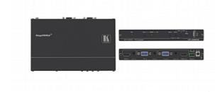
VP426H2 is a highperformance digital scaler for HDMI and computer graphics/HDTV signals. The unit up or downscales computer graphics and HDTV signals to resolutions up to 4Kx2K. 28 output resolutions and native are supported. The user selects the computer graphics/HDTV or HDMI input and the scaled output is sent to both the computer graphics and HDMI outputs
