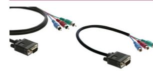
Kramer's CGM/3RVF is constructed from 3 mini coax cables with a 15pin HD (M) connector at one end and 3 RCA (M or F) connectors at the other. These cables send or receive computer graphics video or component video signals
