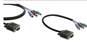
Kramer's computer graphics video to component video breakout cables are constructed from 3 mini coax cables with a 15-pin HD (M) connector at one end and 3 RCA (M or F) connectors at the other. These cables send or receive computer graphics video or component video signals
