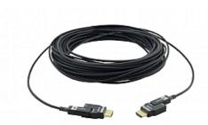
The CP-AOCH/60 is an innovative active optical HDMI cable for 4K@60Hz (4:4:4) signal resolution up to 100 meters (328 ft). This hybrid-fiber cable features micro-HDMI ends with detachable HDMI connectors, making it easy to run through a conduit or other tight spaces. Detachable DVI connectors can be purchased separately.
