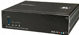
KDS-10 is an advanced, dual stream transceiver for streaming 4K@60Hz (4:4:4) video signals via Ethernet over copper cable. KDS-10 can be set as either an encoder or decoder. As an encoder, it encodes and streams one or two HDMI inputs over an IP network. As a decoder, it receives the encoded signal, decodes it and outputs it to an HDMI output
