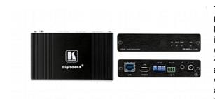
TP-583Txr is a high-performance, extended-reach HDBaseT transmitter for 4K HDR HDMI, RS-232 and IR signals over twisted pair. TP-583Txr converts all input signals into the transmitted HDBaseT signal. It enables extending video signal up to 100m (330ft) at 4K@60Hz (4:4:4) video resolution, up to 180m (590ft) at 4K@30Hz (4:4:4), and up to 200m (650ft) at HD video resolution over Kramer copper cables. It is compatible with standard HDBaseT-compliant extenders at 4K@30Hz and HD video resolutions
