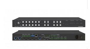
VS-622DT is an all-in-one 4K@60Hz (4:2:0) presentation system with 6x2 HDMI/HDBaseT matrix switching, control gateway, PoE, power amplifier, and Maestro room automation. The unit reclocks and equalizes the signals and can route any input to the HDMI or the HDBaseT output or to both outputs simultaneously. It supports resolutions up to 4K@60Hz (4:2:0) and WUXGA.
