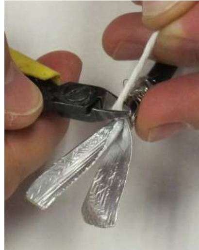
Figure (10): Removing the filler
