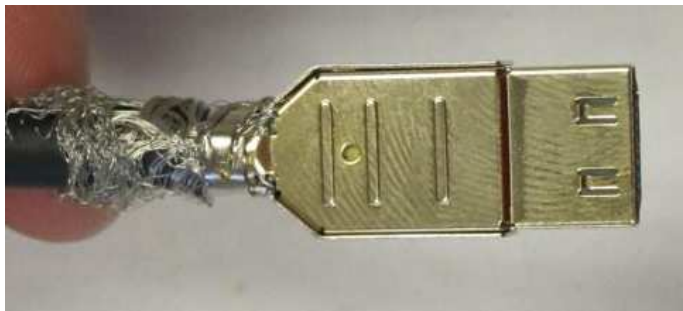
Figure (32): Properly crimped strain relief
