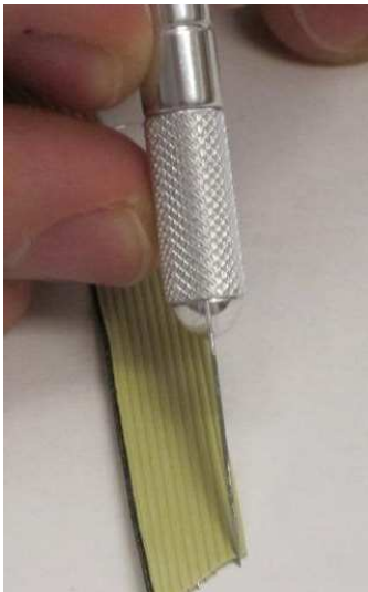
Figure (15): Outer Conductor stripped
