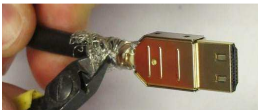
Figure (33): Trimming braid shield
