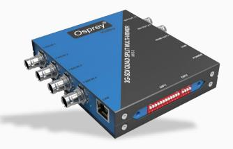
One or more inputs can be scaled and directed to the outputs in a variety of layouts. All inputs are resolution and frame rate independent. In addition, audio bars can be overlaid on each channel for quick signal monitoring. Text overlay can be customized for each input and as an additional feature input resolution display can be enabled or disabled.
