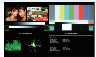
Dual 3 Gb/s Input Display Mode SDI-1, SDI-2, Waveform / Vectorscope, 16 CH Audio Level Meter, VPID & Time Code
