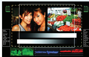
Advanced Waveform + VPID + Marker SDI-1, Waveform, (Y,Cr,Cb), 16 CH Audio Level Meter, VPID & Marker
