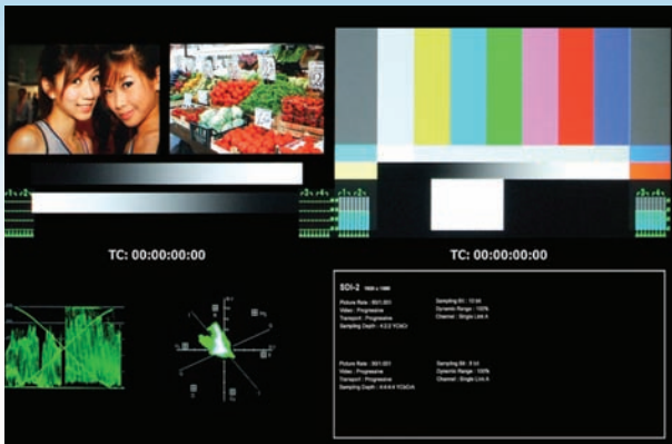
Dual Display Mode with Waveform & Vector
