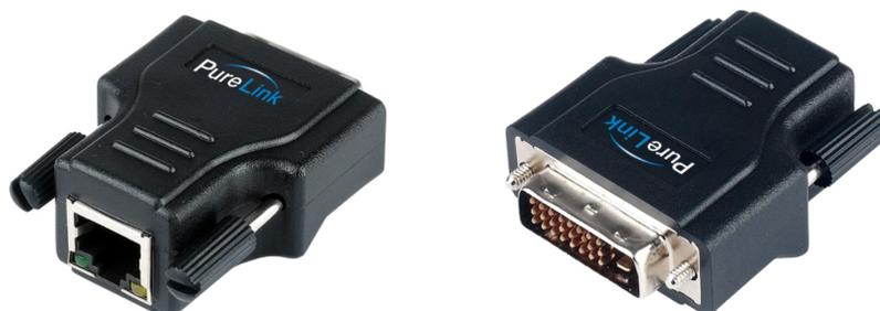
The **DCE II Tx/Rx** DVI over CATx Extension System provides reliable transmission and extension of Full-HD video from a DVI source using a single CATx cable. With support for resolutions up to 1920×1200 at distances of 165 ft. and 1024×768 at distances of 220 ft., along with embedded EDID and device recognition, the DCE II Tx/Rx offers a convenient video extension solution ideal for any small-scale, point-to-point presentation or digital signage application.
