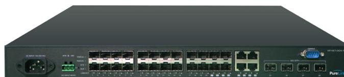
The **VIP-NET-0424-1G Media Hub** is a next-generation L2+ managed fiber switch purpose-designed for AV over IP applications. The VIP-NET-0424-1G offers a full suite of L2 features, including advanced L3 functions such as Static Rout, that deliver better performance via fiber or copper connections and lower total cost of ownership in Enterprise networks.
